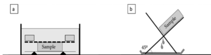
Fig. 1. Water absorption test of biocomposite (Salas-Ruiz, 2019)
